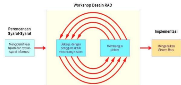
Gambar 2. Tahapan Metode Rapid Application Development (RAD)
